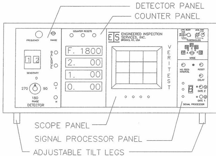
**SENSORS:** Coils are available in sizes from  $\frac{1}{4}$ " through 6" i.d. in roughly  $\frac{1}{4}$ " increments (circular or rectangular configurations); special sizes can be manufactured. Probes of any specified o.d. are also available.
